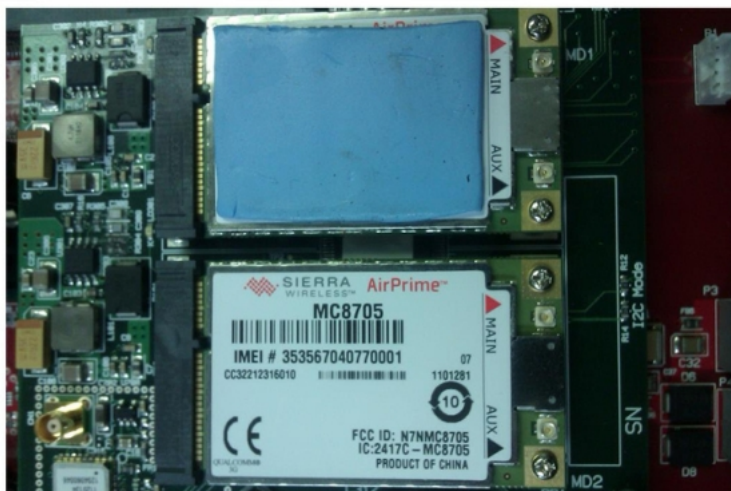
Fig. 11: Example of a Thermal Pad assembled over the WWAN MD1. This must be assembled in both.
