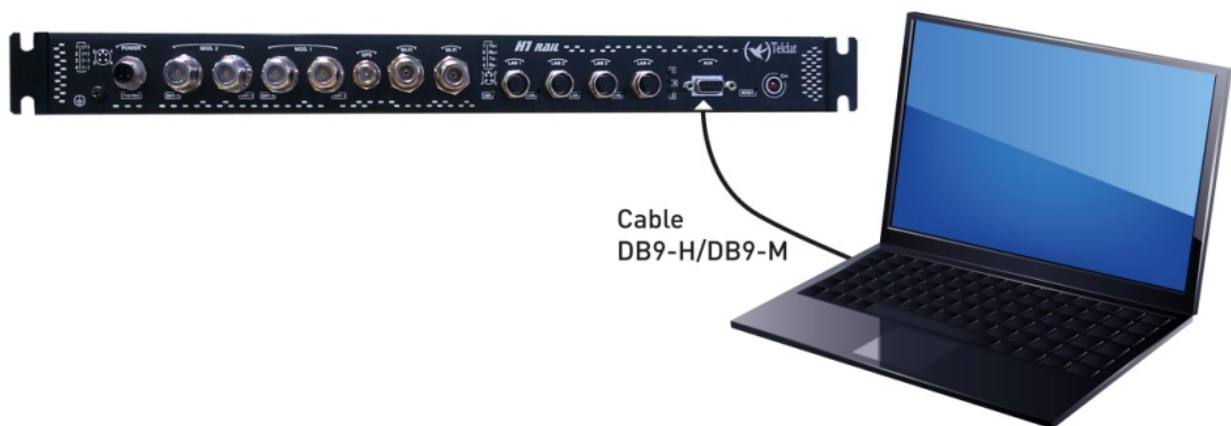
Fig. 8: Connection for configuration
